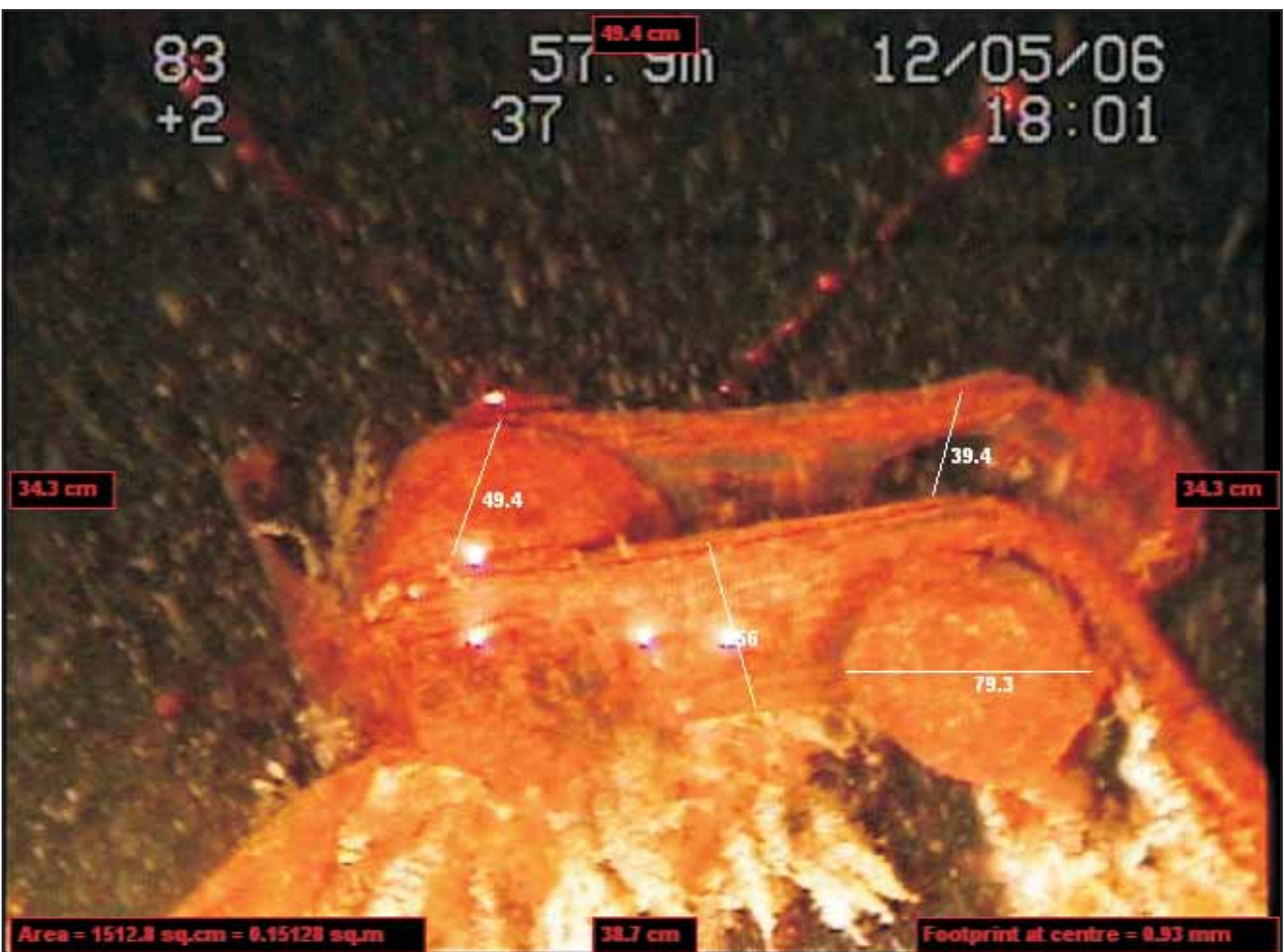
Plate 2: Scaling camera shot of the same fastening.
