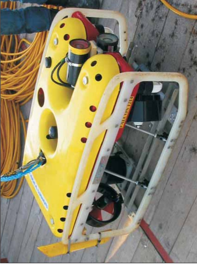
Plate 3: SCOUT transponder mounted on the ROV.
