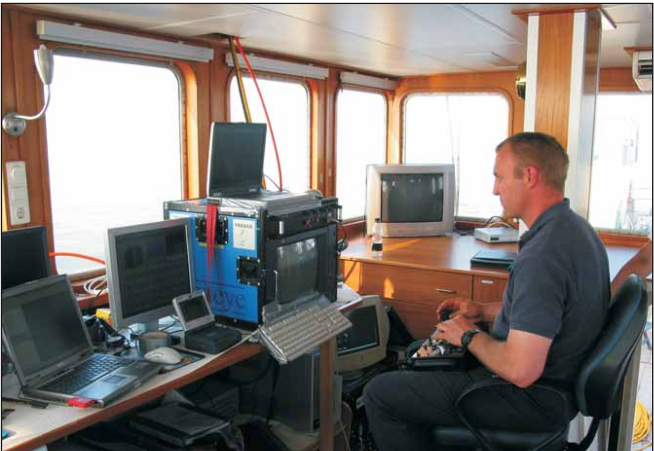
Plate 2: ROV control system set up in the wheelhouse of Sara Maatje XV .
