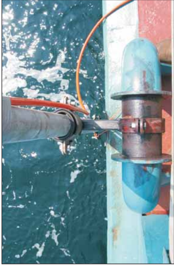
Plate 2: SCOUT transceiver on pole.
