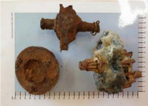
Brett\_1032 was identified by Steve as parts from a BMW 801. This particular engine was fitted to three types of aircraft that operated over the UK. These being the Focke-Wulf 190 fighter, the Dornier 217 bomber and the Junkers 88.
