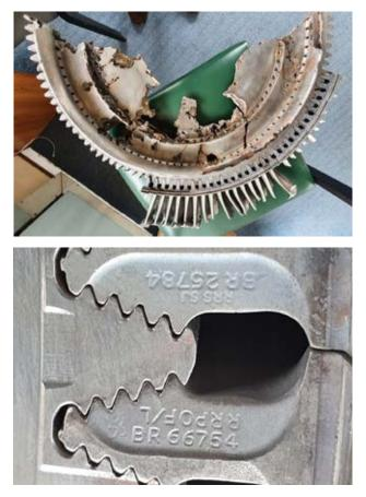
**Top:** Tarmac\_0988, a metal engine part from a Rolls-Royce Avon engine; **Bottom:** the 'RR' mark used to identify this piece.
