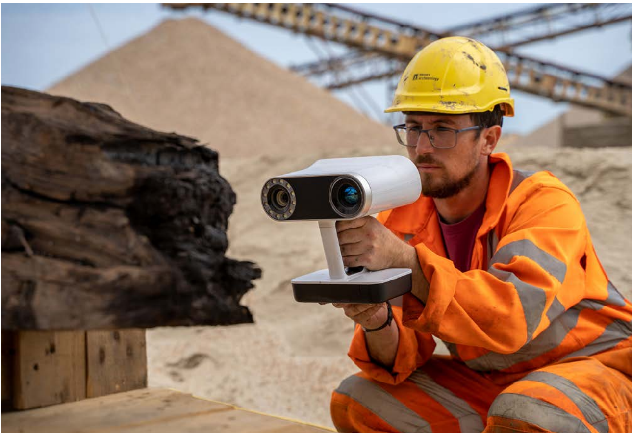
Specialist Paolo Croce (Wessex Archaeology) recording the timbers of the Dungeness Wreck using an Artec 3D scanner
