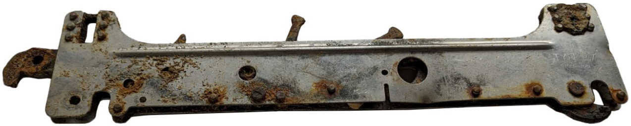
Britannia_1074, a B7 bomb shackle, identified based on the reference marks [TYPE-B-7] [100-1100] and [FRONT]
