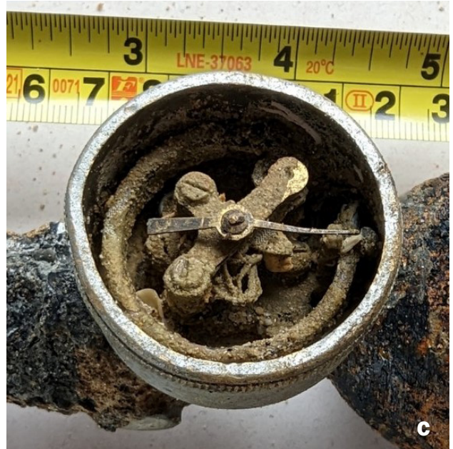
A, B and C, above: Britannia_1073 , a small gas cylinder with valve and gauge, discovered by Dean Jackson and Robert Lockley on board Britannia Beaver . The letters [..HOHEM..] and [..AND] are visible on the neck of the valve
