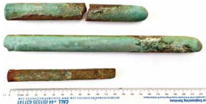
Plate C12: ships pins recovered from the Eriskay site and reported to the Receiver of Wreck under DROIT No 001/13 (© A. Hunt 2016)
