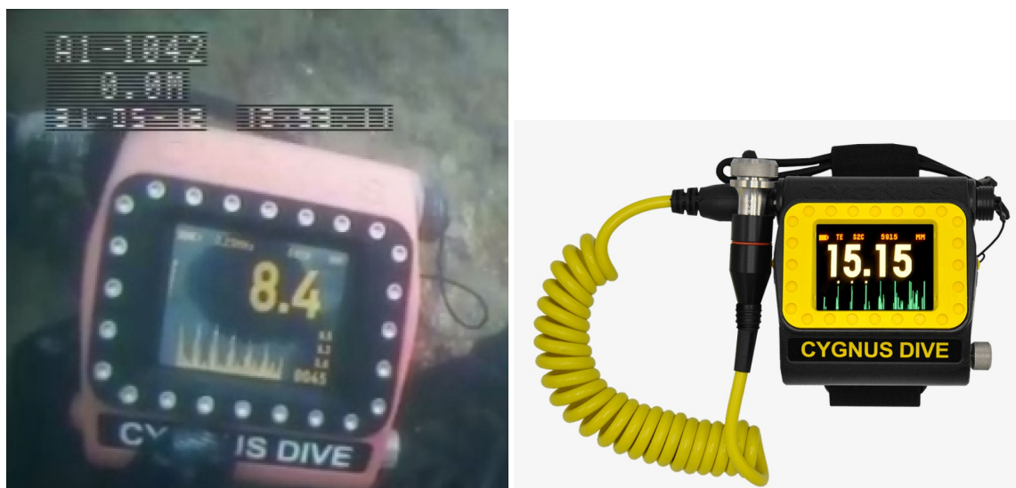
Thickness measurement of the pressure hull of the A1. The probe is being held against the bare metal of the hull plating behind the wrist monitor. The image on the right shows a similar gauge and probe on the surface.
