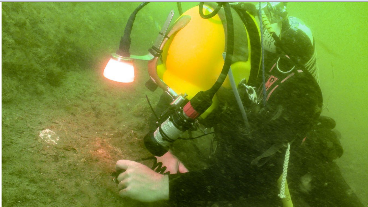
Surface supplied diver taking a UT measurement of the A1 hull through a small hole in the concretion.
