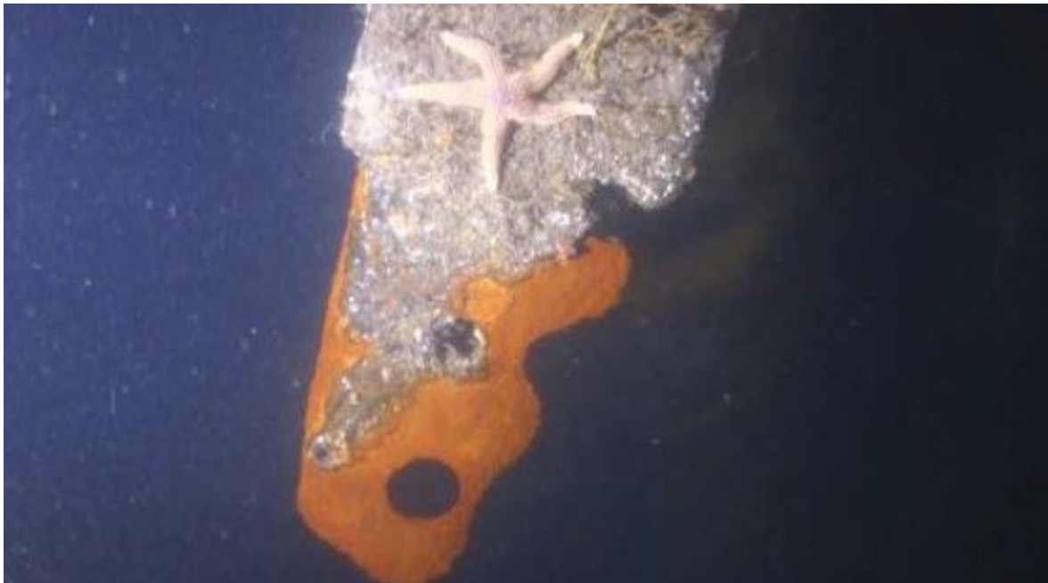
UB-107 off Flamborough Head. Active corrosion of the damaged hull above the Forward Battery Compartment. The corrosion layer formed by fouling and oxide has spalled off, possibly as a result of a recent impact. This has exposed the surface of fresh steel, which has begun oxidising and is an orange colour in the diver's torchlight.
