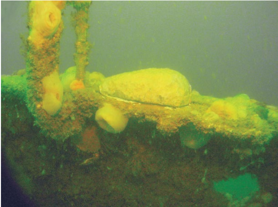
Sacrificial anode attached to the top of conning tower of the very early Resurgam submarine off North Wales in 2006
