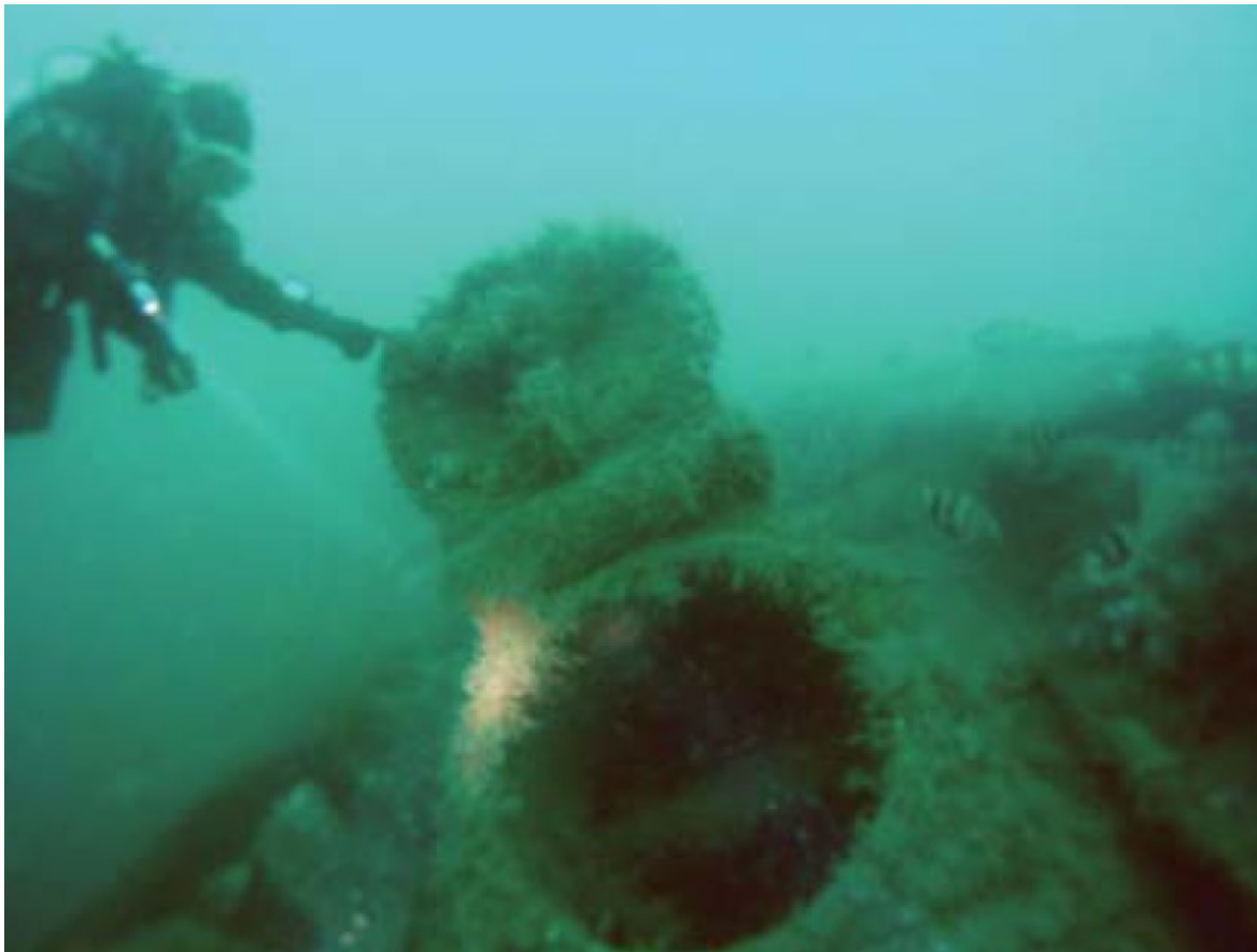
Aft loading hatch of the UB-78. The angle of the hatch relative to the top of the pressure hull indicates that it is for loading torpedoes.
